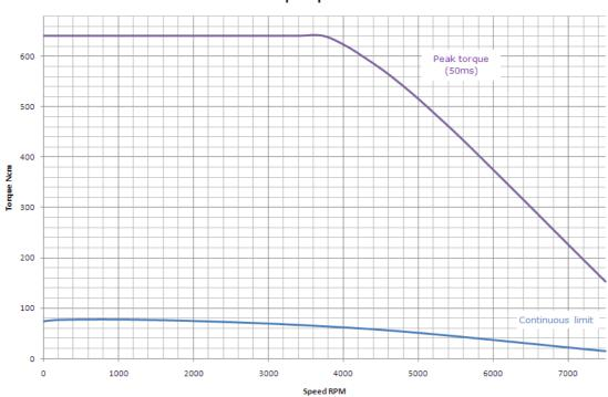
NOTE: The angle of the Torque/Speed curve remains the same for higher and lower voltages. The speed varies proportionally from zero rpm relative to the voltage supplied. The stated voltage is an example, not a predefined maximum or minimum. Due to ongoing product improvement data in this datasheet maybe subject to change without notice.
